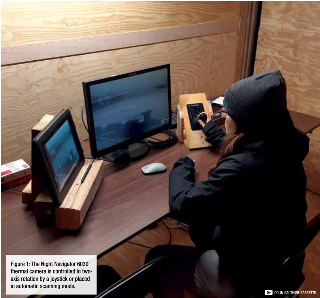
Figure 1: The Night Navigator 6030 thermal camera is controlled in two-axis rotation by a joystick or placed in automatic scanning mode.
